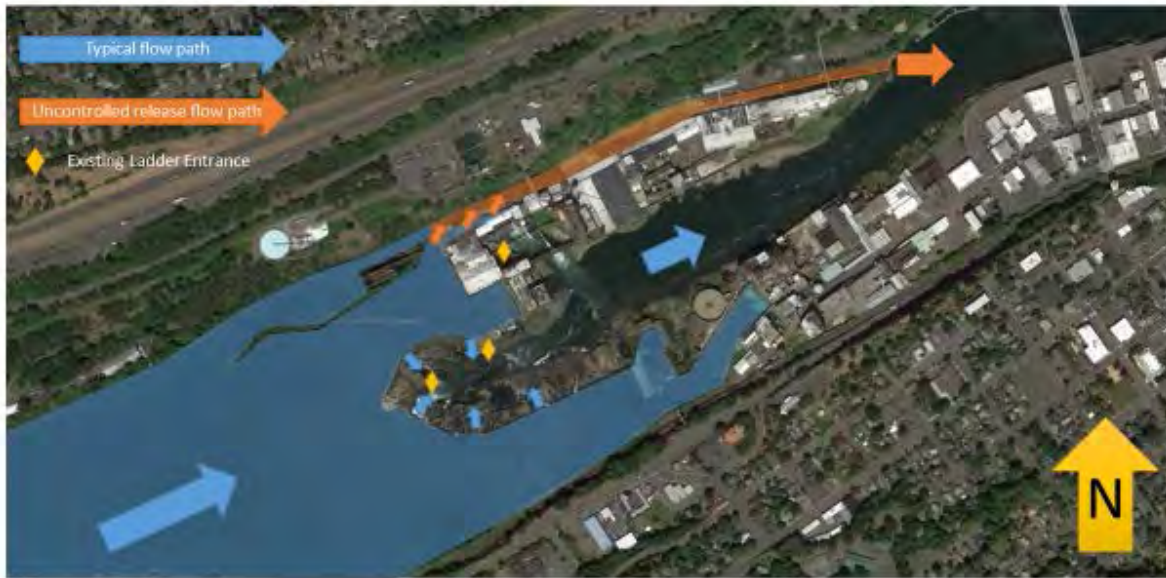
Figure 16: Flow path developed during an uncontrolled release through the Willamette Falls Locks.
