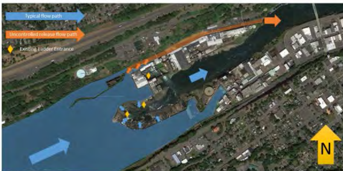
Figure 28. Flow path developed during an uncontrolled release through the Willamette Falls Locks.
